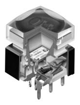
Compact miniature pushbutton has two-point pressure that insures secure lock structure. A hook pin that locks the cap is held using an elastic plate. By holding cap from both above and below, a stable lock results that resists vibration and damage from impact.
